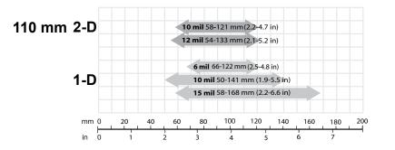
The following table shows the Field of View widths in mm at various distances.
