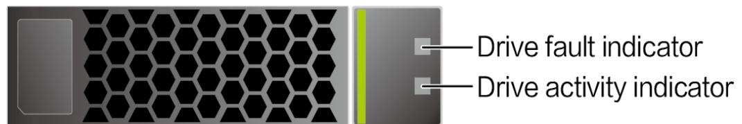
Figure 2-8 Indicators of a 2.5-inch SAS/SATA drive
