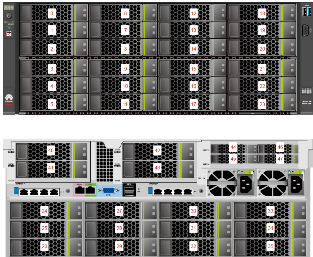
Figure 6-3 Server with 36 x 3.5-inch drives in Expander mode
