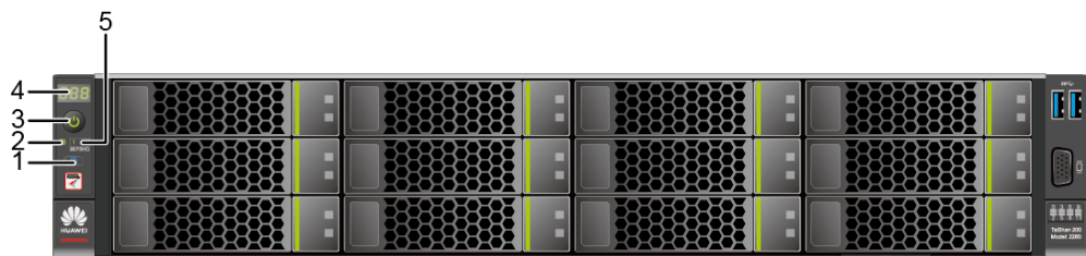
Figure 4-7 Indicators and buttons on the front panel of a server with 12 x 3.5-inch drives
