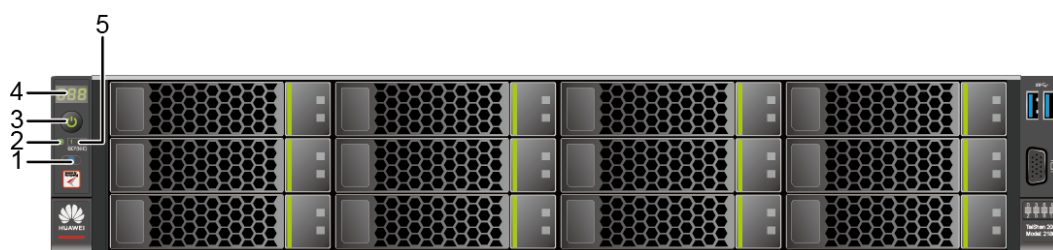
Figure 4-4 Indicators and buttons on the front panel of a server with 12 x 3.5-inch drives
