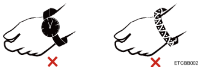
Figure 8-2 Conductive objects to be removed
