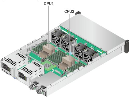
Figure 5-19 Processor positions
