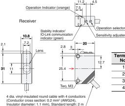
4 dia. vinyl-insulated round cable with 4 conductors (Conductor cross section: 0.2 mm² (AWG24), Insulator diameter: 1.1 mm), Standard length: 2 m
